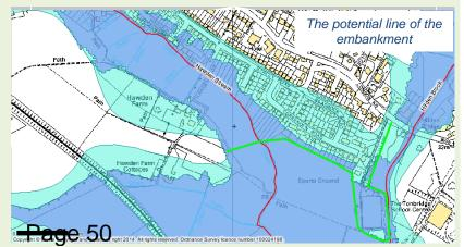
to pump water from the Hawden Stream onto the sports pitches will need to be included. Design will take place over the winter and spring. Construction is planned to take place in summer 2015.
